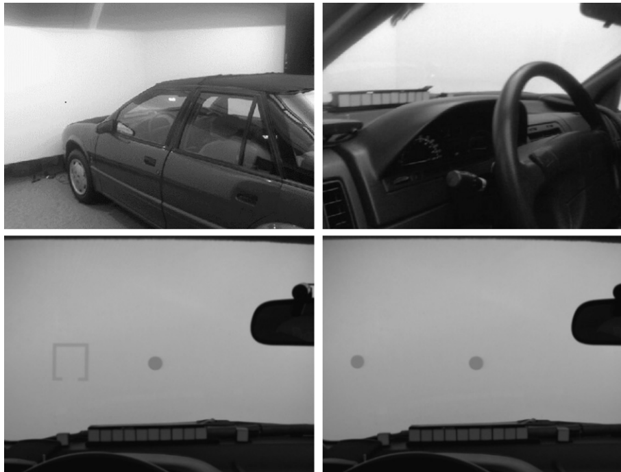
Fig. 1. Participants sat in the driver's seat of the SIREN simulator (top left) and viewed targets (bottom left) and either extra-vehicular cues presented on the center screen (bottom right) or in-vehicular cues. The top right image shows the implementation of the LEDs for the in-vehicle visual cues and the flat speakers for the auditory cues placed inside the vehicle cab.
